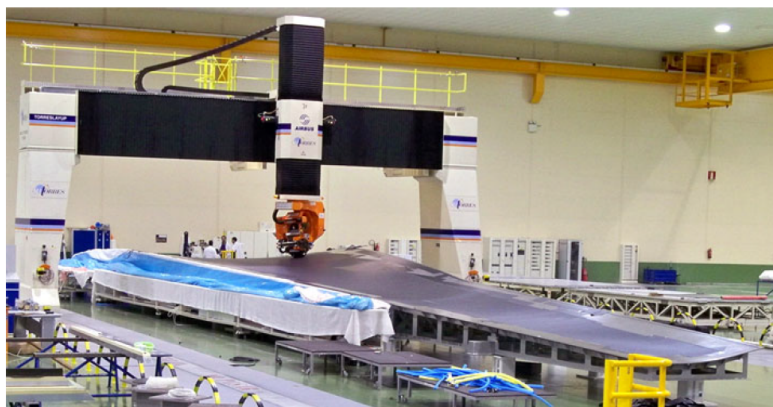
Figure 2.8: M-Torres TORRESLAYUP machine manufacturing a wing skin [59].
