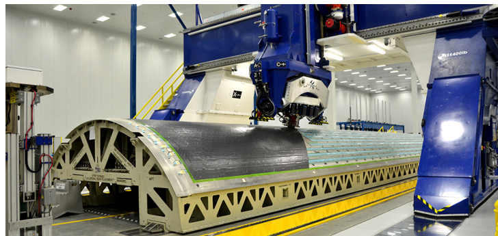
Figure 2.10: Electroimpact AFP gantry machine manufacturing a fuselage panel [75].
